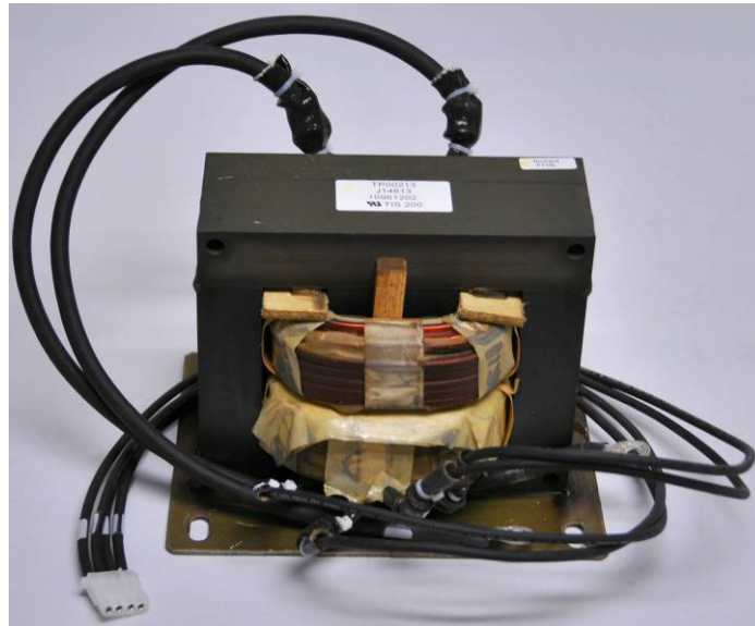
Figure 6: Inverter & Voltage Regulation Transformer
