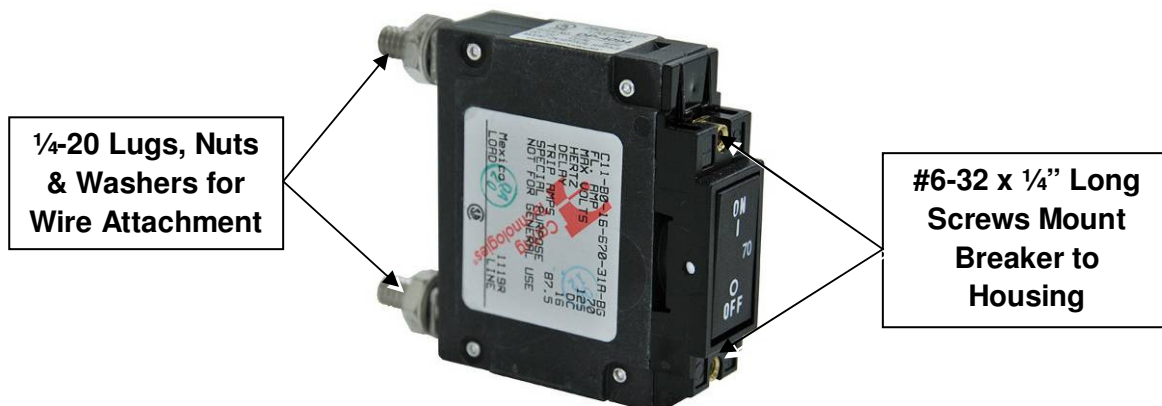
Figure 10: DC Circuit Breaker
