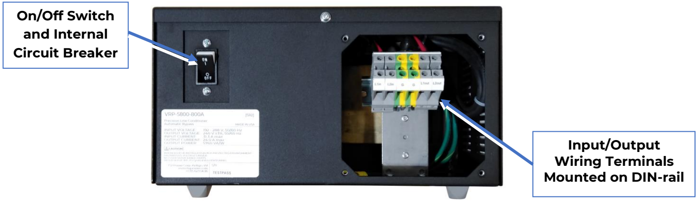
Figure 8: Small Series VRP Shown With Rear Access Cover Removed
