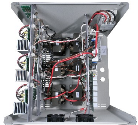
Top view showing the internal components (VRP-45000-8775 shown)
