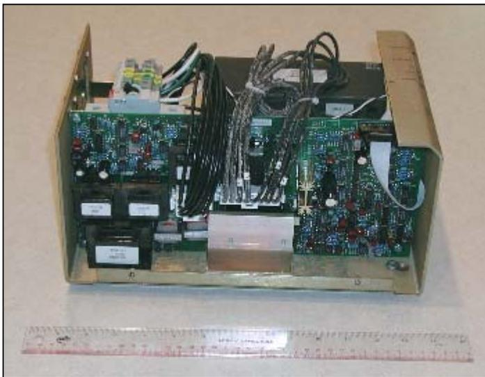
The VRe is capable of providing regulated output while operating over a wide input range of 160VAC to 330VAC. Unlike most existing power conditioners, the VRe is specifically designed to handle this wide range of input voltage at full rated power over the entire specified operating temperature range.
