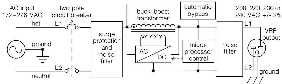
**Figure 5:** High-speed VRP PWM (pulse-width-modulation) AVR.
