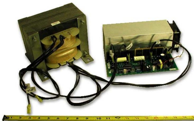
**Plate 1:** 7500 VA single-phase system with buck-boost transformer and heatsink-pcb assembly. Note: ruler scale in inches.
