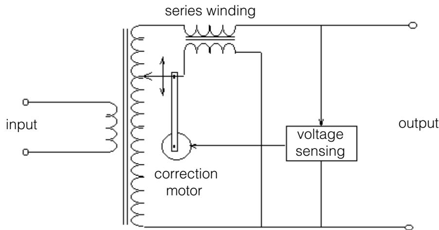
Figure 2: Electromechanical servo AVR.
