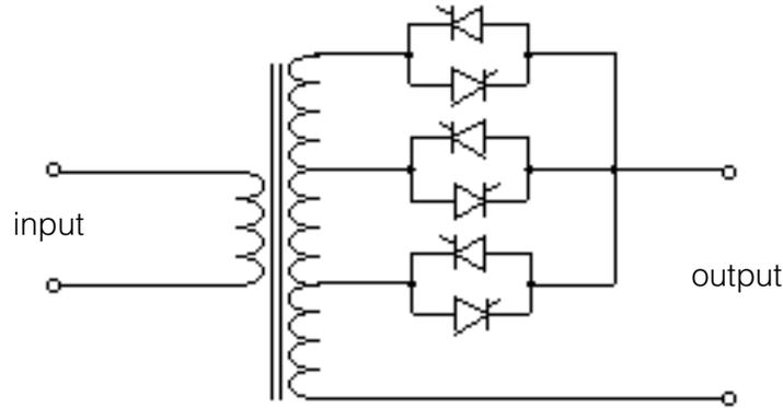
**Figure 3:** Electronic tap-switching AVR.
