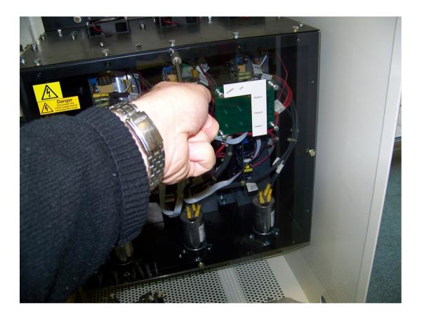
Remove all fast-on terminals from PCB. Begin with front five (5) terminals. Then remove seven (7) terminals closest to heatsink.
